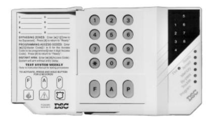
PRESS [F] for 2 seconds to activate FIRE transmission.
