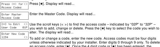
unless otherwise indicated by your installer. Enter digits 0 through 9 only. To delete an access code, enter [\*]. Once the 4 digit code or [\*] has been entered, the keypad sounder will beep 3 times and the display will read...
